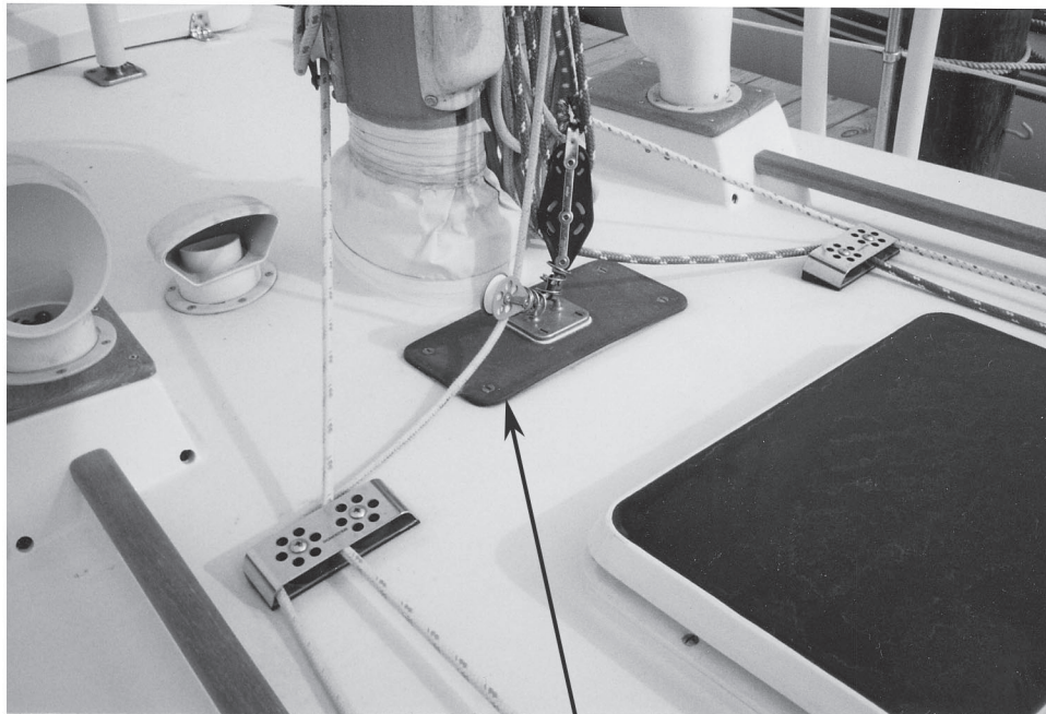
The 1/4" aluminum plate is installed just aft of the mast partners. The padeye on top of the plate anchors turning blocks used for running various lines back to the cockpit. In this current "cruising" configuration these are a single-line 1st reef (to port) & the mainsail cunningham (to stbd) . Other lines running back to the cockpit are the main halyard (port) and the spinnaker pole topping lift (stbd); these lines go through turning blocks mounted on the mast, just above the partners.
